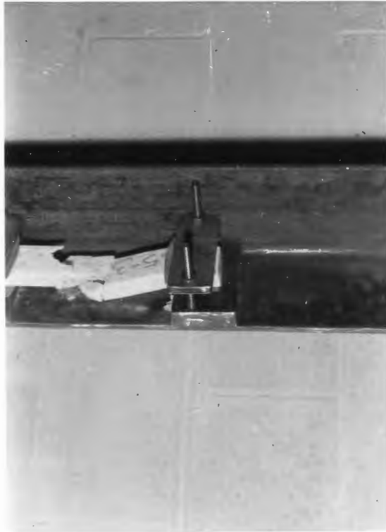
Fig. 18 Broken Gypsum Beam After Test.
